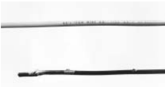
After two years underground, buried THHN (bottom) shows much deterioration. The PE insulated material, on the other hand, stood up very well.
