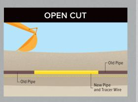
Open cut trenching is the traditional method for excavation used to expose existing or install new utilities where there are no buildings or other obstructions, then backfilling the trench.
